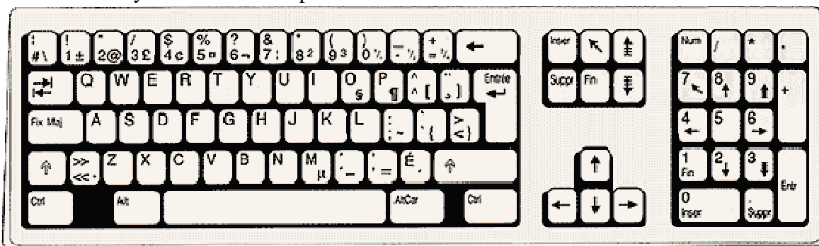
French Canadian Keyboard - to access symbols on right of key press right Alt key and letter key. Example: Right Alt + 2 gives the @ symbol
